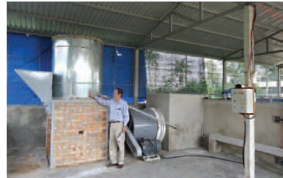
Mr. Thai Van Quang, National Project Coordinator, by the burner of the dryer
